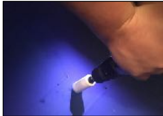
Figure 30 Drill the center of the mark out with a drill bit.
