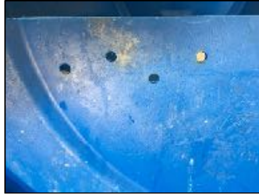
Figure 20 Use a drill bit to make holes
