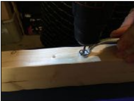
Figure 28 Make holes for the screws of the handle
